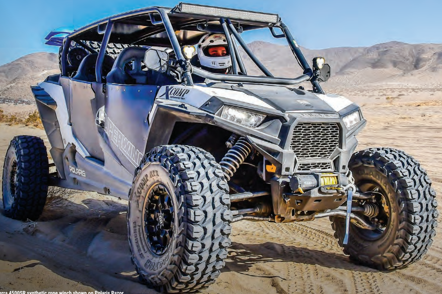
Terra 4500SR synthetic rope winch shown on Polaris RZR
