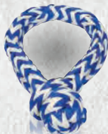
SOFT SHACKLE 1/2" Soft Shackle. 30,000 Load Rating. 38,000 lbs. Breaking Strength. Part No. 2574
