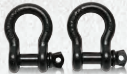
3/4" BOW SHACKLE (2) 3/4" with 7/8" diameter pin; 10,000 lb. capacity Part No. 2538
